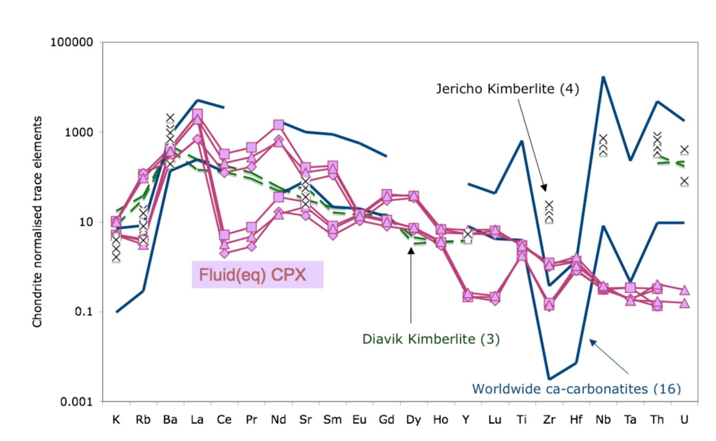
The composition of the fluids in equilibrium with the metasomatised CPX rimming carbonatite (rhombus), calice-silicate (triangle) and calcitebearing silicate (square) was calculated using  $D_{(CPX/Melt)}$  values from the literature (6-11). The results show similarities with the composition of kimberlites (3, 4) and worldwide Ca-carbonatites (16), , except for lower Nb, Ta, Th and U.
