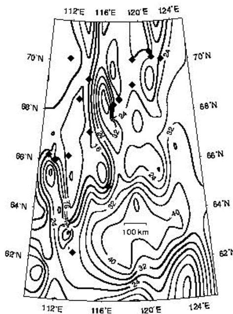
Figure 1. Effective elastic thickness contour map of the Siberian platform. Contour interval 4 km. The black diamonds represent the kimberlite fields where mantle material was analysed to construct mantle sections.
