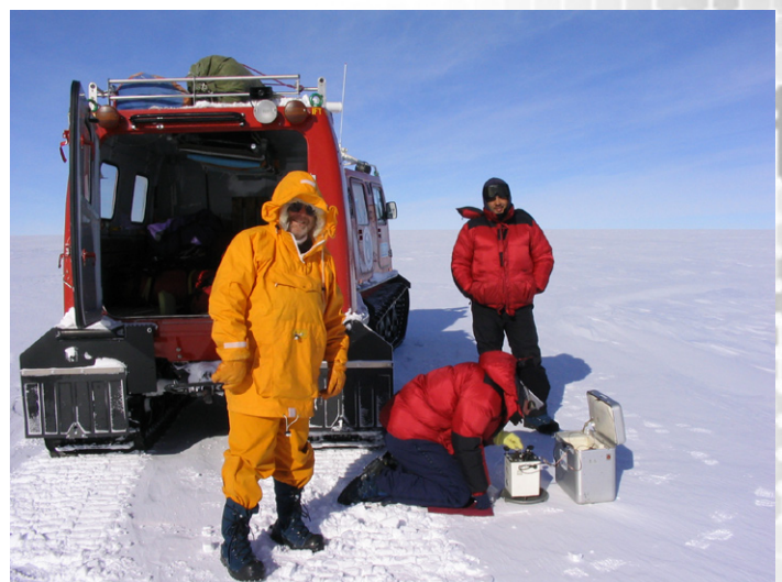
Taking a gravity measurement on the Law Dome ice cap along side a Hagglands tracked vehicle.
